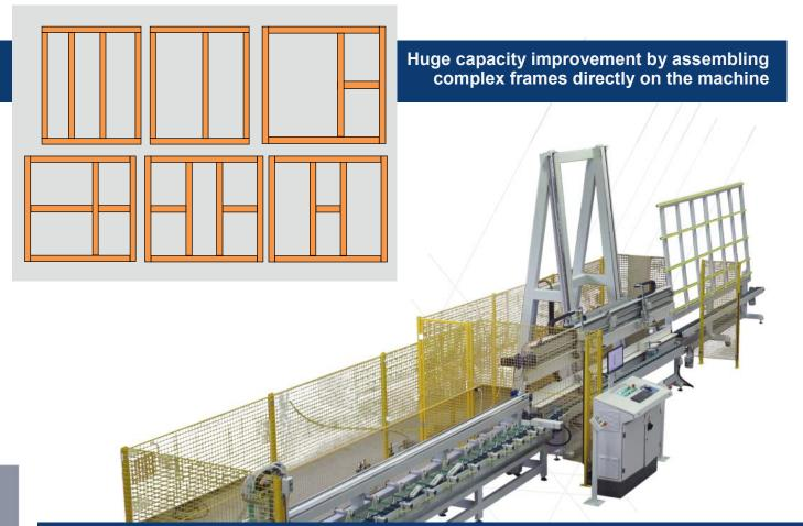
Assembling process efficiency improved by integrating automatic gluing 4Glue-L and TITANPRESS-TX
